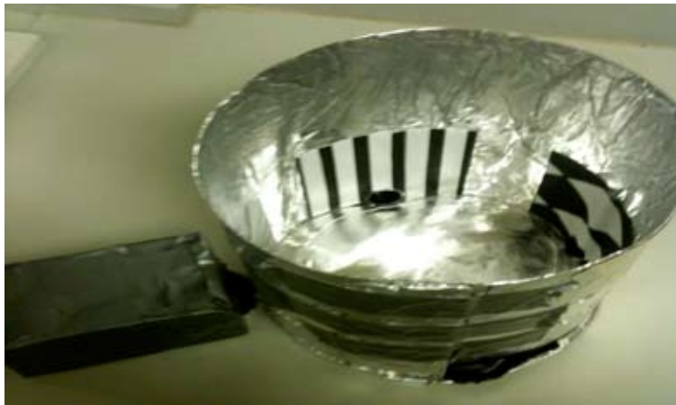
The modified Barnes maze consisted of a 12-inch circular aluminum platform surrounded by a 10-in aluminum wall. Overhead heat and light was used to motivate the subjects to find the real exit among the 3 false exits.
