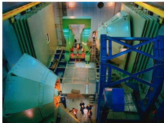
Figure 4. This figure shows a very empty 'intersection region' looking west. A central magnet is surrounded on the sides by two larger muon magnets. When operational, researchers will fill the carriage in the foreground with detectors.
